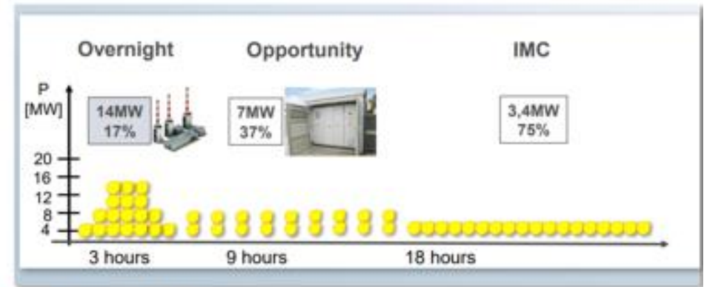
Charging power of a E-Bus fleet (100 vehicles) 18m Buses
